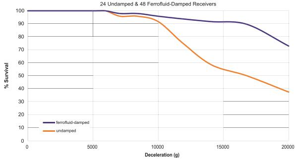
**Figure 8:** Percent of surviving ferrofluid-damped and undamped ED receivers for increasing drop height.
