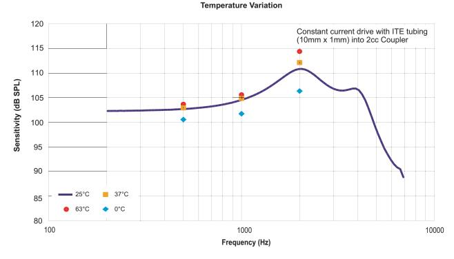
Figure 7: Frequency response of an FED receiver at temperatures: 0°C, 25°C, 37°C, and 63°C.
