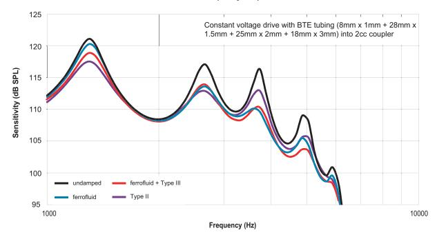
**Figure 6:** Frequency response of damped and undamped ED receivers connected to BTE tubing and a 2cm<sup>3</sup> coupler cavity under constant voltage drive conditions (magnified view).
