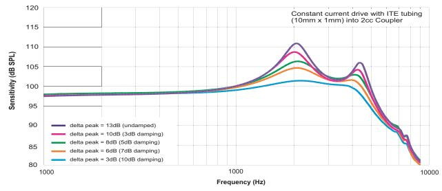
**Figure 3:** Frequency response curves under constant current drive conditions for fluid-damped FED receivers and a response curve for an undamped ED receiver. Labels in legend are the delta peak values.
