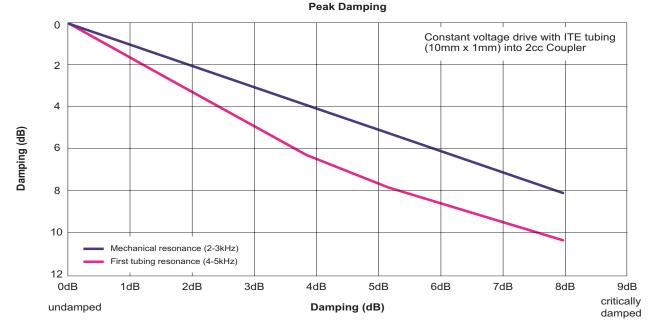
**Figure 4:** Damping for the first and second peaks in the frequency response of the FED receiver connected to ITE tubing and a 2cm<sup>3</sup> coupler under constant voltage drive conditions.
