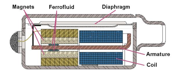
Figure 1: Cross-section of the Knowles FED receiver (i.e., ferrofluid-damped ED receiver)
