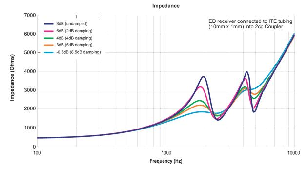
**Figure 11:** Impedance curves for fluid-damped and undamped ED receivers connected to ITE tubing and a 2cm<sup>3</sup> coupler. Labels in legend are the delta peak values under constant voltage drive conditions.
