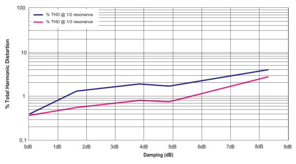
Figure 10: Percent of total harmonic distortion at 1/2 and 1/3 resonance versus damping under constant voltage drive conditions (FED receivers).
