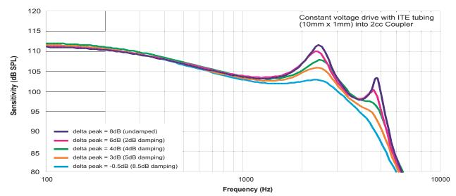
**Figure 2:** Frequency response curves under constant voltage drive conditions for fluid-damped FED receivers and a response curve for an undamped ED receiver. Labels in legend are the delta peak values.
